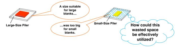
[Countermeasure] A single piler that could accommodate both single and dual piling was installed.
